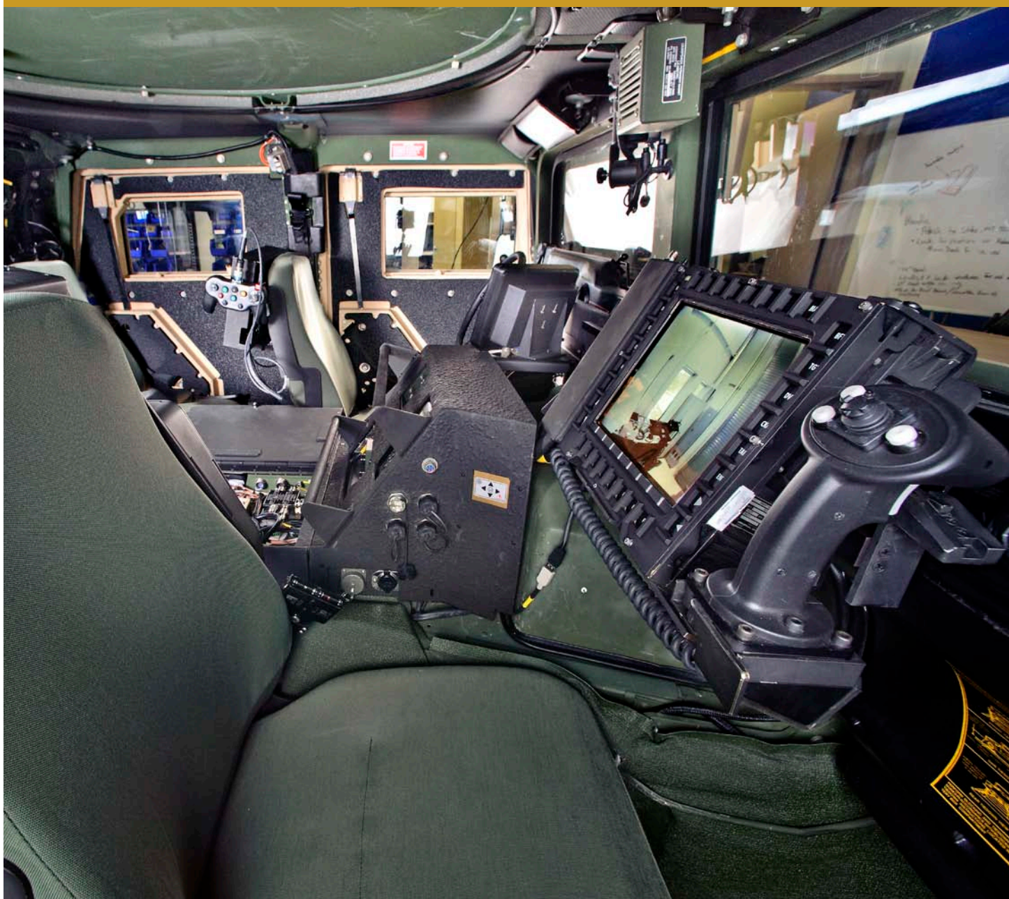
Pictured is an interior view of a four-seat Up-Armored M1165 HMMWV that uses a vetronics system from General Dynamics C4 Systems that leverages an Open Systems Software Framework and embedded small form factor hardware.
