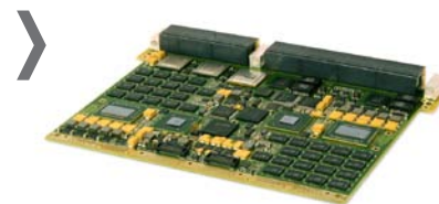
Figure 1 | DSP280 rugged, dual-socket, Intel second-generation quad Core i7 multiprocessor from GE Intelligent Platforms
